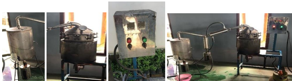
Gambar 1. Kondensor, Control Panel, Rangkaian Alat Pyrolisis
